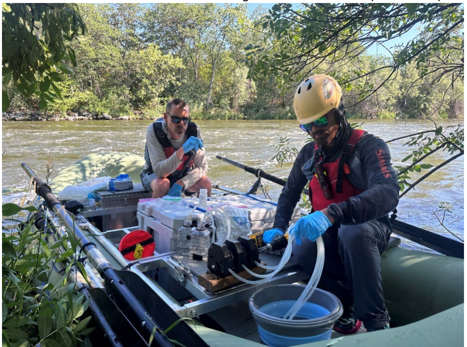
Figure 1: RES staff filter genetic material from water samples using peristaltic pumps at a boat access monitoring site along the Klamath River.
